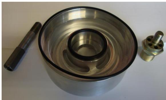
This filter adaptor is intended for the Jaguar XK140 and MkVII/VIII/IX models fitted with a Tecalemit filter head FA2708 – the name Tecalemit will be found cast in to the left hand side of the filter head. As it is common to find the filter head from one Jaguar engine fitted to another please check that you have the correct adaptor for your engine. Check the engine numbers below or contact your supplier if in doubt.
